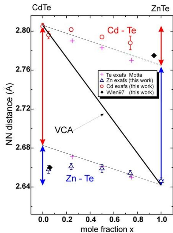
Fig. 2: Local bond length of Cd – Te (circles) and Zn – Te (triangles). The local bond lengths deviate strongly from Vegard's law (VCA) as given by x-ray diffraction data [1] and are significantly less than a quarter of the bond-length difference of the pure systems (compare the arrows). Calculated values (WIEN97, diamonds) support the experimentally observed strong local nature of the cation-anion bond.
