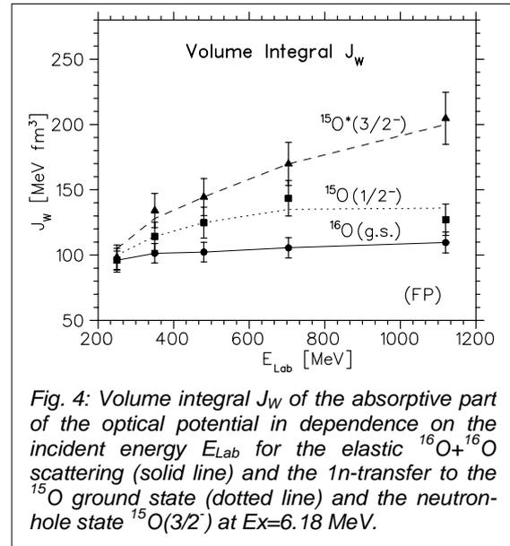
Fig. 4: Volume integral  $J_W$  of the absorptive part of the optical potential in dependence on the incident energy  $E_{\text{Lab}}$  for the elastic  $^{16}\text{O}+^{16}\text{O}$  scattering (solid line) and the  $1n$ -transfer to the  $^{15}\text{O}$  ground state (dotted line) and the neutron-hole state  $^{15}\text{O}(3/2^-)$  at  $E_x=6.18$  MeV.
