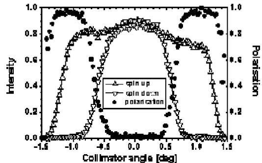
Fig. 2 Transmission coefficient for the two spin states for neutrons with a wavelength of  $4.72 \text{ \AA}$  through a radial collimator channel formed by Si wafers coated with a FeCo-Si supermirror followed by a Gd layer, measured in a magnetic field of 300 Oe.
