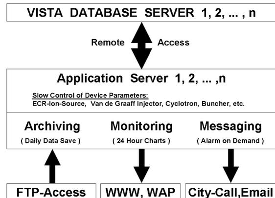
Fig. 3: Linux Application Server supporting the monitoring of the ISL-Facility.
