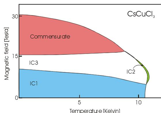
Fig. 2: Magnetic phase diagram of CsCuCl<sub>3</sub> with the field in the *ab*-plane. IC1, IC2, and IC3 indicate different incommensurate structures. The structure of phase IC2 was studied earlier [2].
