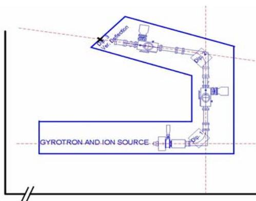
*Fig. 5: Injection Line for a superconducting ECR Ion Source
