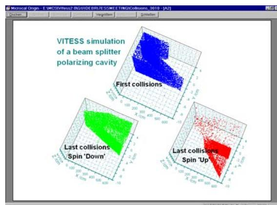
Fig. 2: Recent Monte Carlo simulations for the optimization of polarizing cavity systems and their application at ESS.
