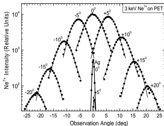
Fig. 2: Angular distributions of  $\text{Ne}^{7+}$  ions transmitted through capillaries in PET. The tilt angle is indicated. Also plotted are data for capillaries in Ag showing that the angular distributions are quite different from those for PET.
