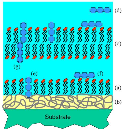
Fig. 1: Schematic diagram illustrating a supported lipid monolayer (a) on a polymer cushion (b) in equilibrium with a free floating lipid bilayer (c) at the solid-liquid interface. Different possible binding sites (e-g) of a water soluble peptide (d) are indicated.
