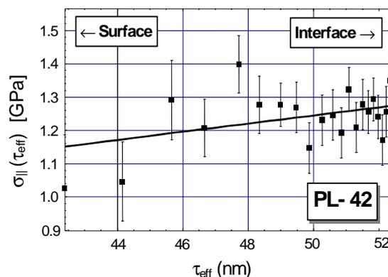
Fig. 2: Depth distribution of the in-plane residual stress  $\sigma_{\parallel}(\tau)$  in a thin boron-doped poly-Si-film (110 nm) deposited on a glass substrate<sup>1</sup>.
