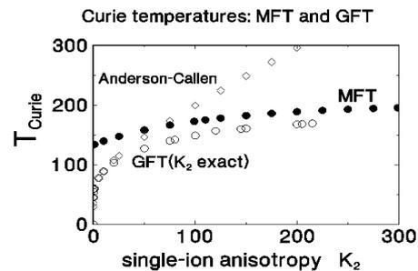
Fig. 1: Comparison of Curie temperatures calculated with the exact (GFT) treatment of the anisotropy terms, the Anderson-Callen decoupling and mean-field theory (MFT).
