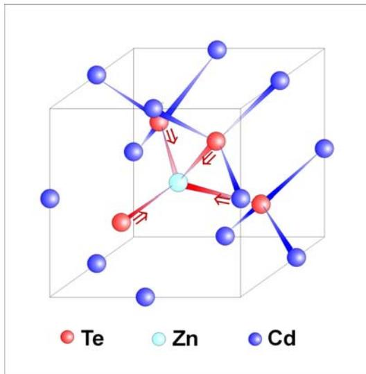
Fig. 1: Illustration of the local lattice relaxation with the incorporation of a Zn atom, replacing a Cd atom in a CdTe lattice. In the case of a Cd atom replacing a Zn atom in a ZnTe lattice the forces are in the opposite direction.
