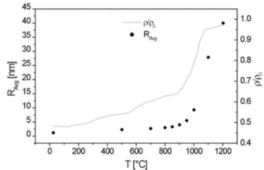
Fig.2: Average particle size  $R_{avg}$ , and relative density  $\rho/\rho_0$  determined by dilatometer experiment
