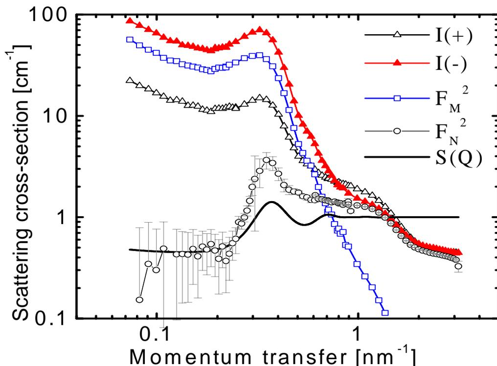
Fig.3: SANS POL intensities  $I^*(Q \perp H)$  (solid triangles) and  $I(Q \parallel H)$  (open triangles) of 5vol% Co-Ferrofluids in  $C_7D_8$  and magnetic (squares) and nuclear (circles) contributions from non-polarized neutrons. The solid line represents the common structure factor  $S(Q)$  for hard spheres.
