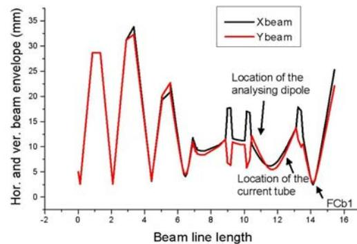
*Fig. 6: The transverse beam envelopes. As indicated, the envelopes show a small beam diameter at the position of the analysis dipole and the tube.*
