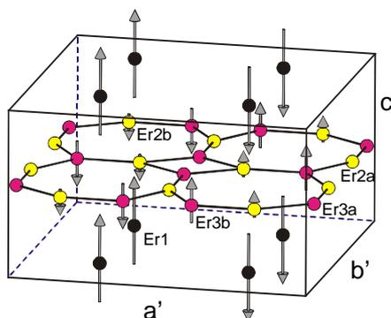
Fig. 1: Magnetic structure model for antiferromagnetic  $\text{Er}_5\text{Ir}_4\text{Si}_{10}$  below 2.8 K as determined by neutron diffraction at BENSC. Only Er ions are shown. The ordered moments are  $|\mu| = 9.0, 1.4, 2.0 \mu_B$  for Er1, 2b, 3b, respectively. For symmetry reasons, the moments on Er 2a and 3a are zero.
