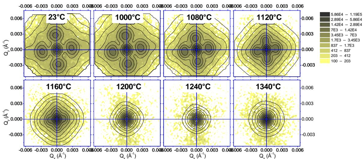
Fig.1: Cross-section in a logarithmic scale for SCA433 superalloy (heat treatment: 1285°C/4h/ air cooling and 1100°C/0.25h/ air cooling) at different temperatures. Color maps are the measured data and the iso-intensity lines denote the fit of the optimum mode.
