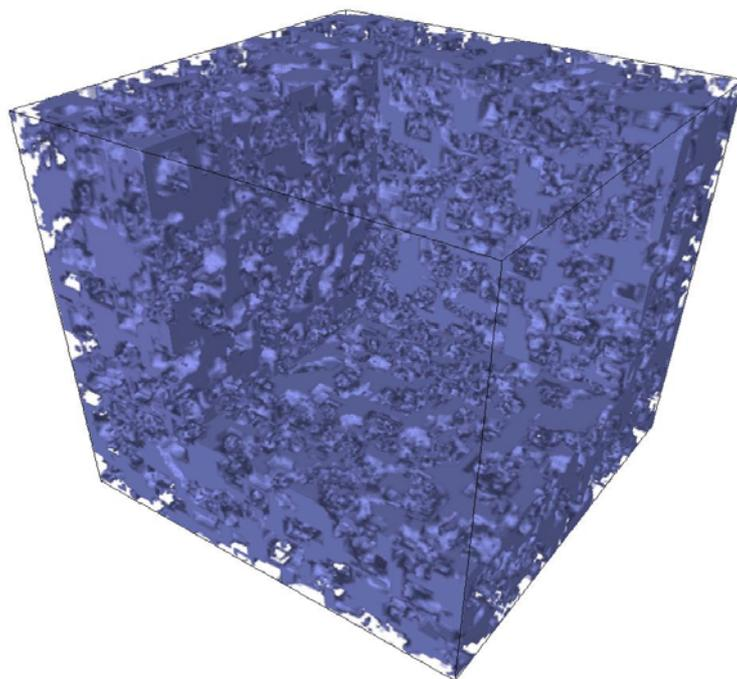
Fig. 2: Binary 3D model of the pore structure as reconstructed by an evolution strategy that adapts the model to the statistical descriptors of Fig. 1. The model uses 1203 bits to represent a Gelsil-50 cube of 80 nm edge-length.
