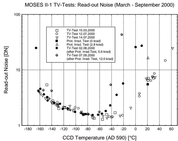
Fig. 2: Read-out noise of the MOSES detector electronics as a function of CCD temperature and increasing total energy doses induced by proton irradiation. Note that the read-out noise returns to normal values at approx.  $-70^\circ\text{C}$  even after 12 krad of radiation of the whole detector electronics including the CCD, whereas at room temperature an increase by more than a factor of 10 can be observed
