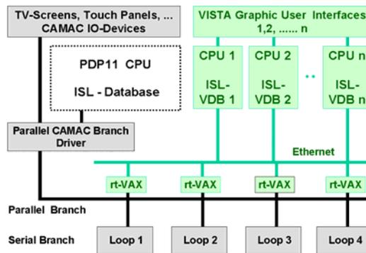
Fig. 1: Schema of the ISL-Control System Upgrade.
