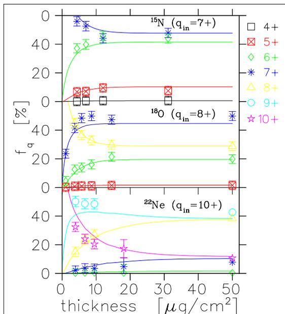
Fig. 1: Evolution of the charge state distributions of  $^{15}\text{N}^{7+}$ ,  $^{18}\text{O}^{8+}$  and  $^{22}\text{Ne}^{10+}$  ions in Carbon at 2 MeV/u in dependence on the layer thickness.
