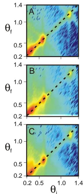
Fig. 3: Diffuse (off-specular) neutron scattering as a function of incident angle  $\theta_i$  and exit angle  $\theta_f$  corresponding to three characteristic fields in the hysteresis loop of the biased state (same as in Fig. 2). Dashed lines correspond to the specular reflectivity shown in Fig. 2.
