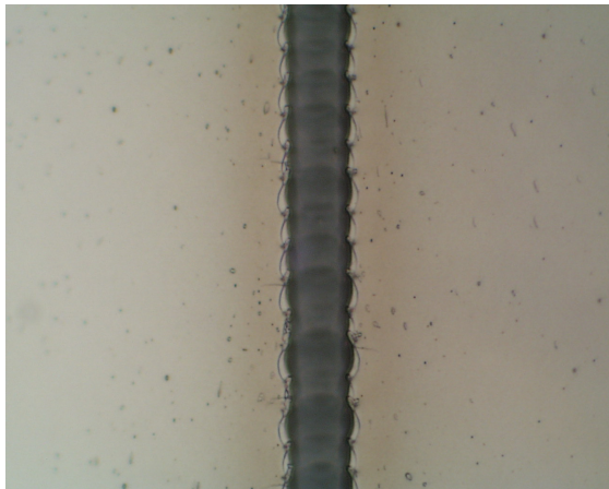
Fig. 1: Molybdenum layer of 1 micron thickness with a laser cut less than 20 micron wide.
