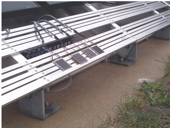
Fig. 4: \text{CuInS}_2 mini-modules at the test array on the HMI campus (near the guesthouse) exposed to the Berlin weather.
