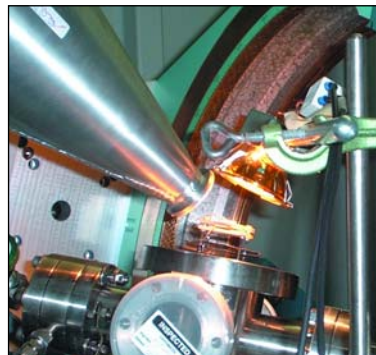
Fig. 3: The sample was mounted on a ceramic holder and irradiated with a halogen lamp. The incoming X-rays entered the figure from the right-hand side. Scattered photons were reflected through the metal cone on the left side to the detector.
