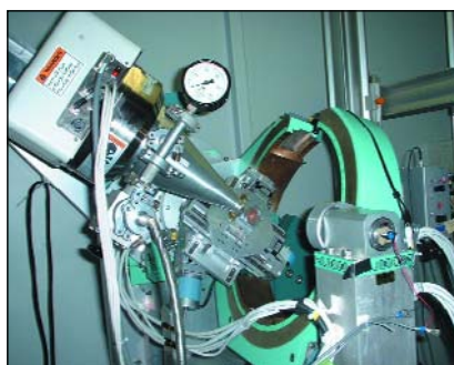
Fig. 1: Improved experimental device used in the investigation of texture changes in thin titanium films with X-rays at BESSY. The figure shows the sample mounted on the goniometer head and the area detector during the measurement. The incoming X-ray beam enters the figure from the right.
