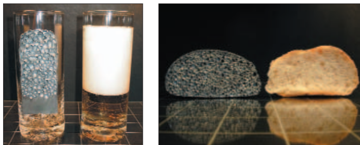
Fig. 1: left: aluminium foam blown with air from a particle-stabilized melt and beer, right: zinc foam and bread roll, both foamed by internal gas creation (Photographs: Hahn-Meitner-Institut)
