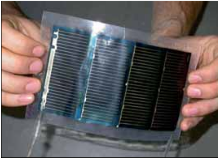
Fig. 2: Encapsulated, flexible CIGSe thin film solar cell module; total area 130 cm 2 and aperture area 108.4 cm 2
