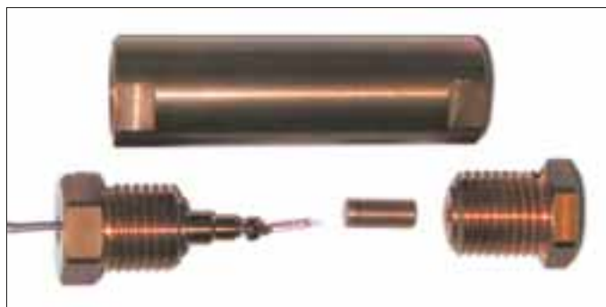
Fig. 2: CuBe clamped cell used in the pressure experiments. Below the main body of the cell from the left to the right: the fixing screw with the manganin pressure sensor and electrical leads, piston and the opposite fixing screw.
