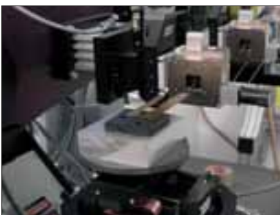
Fig. 2: The brass tongues from a baroque organ during the investigation at the EDDI beamline operated by the Hahn-Meitner-Institut at the synchrotron radiation source BESSY
