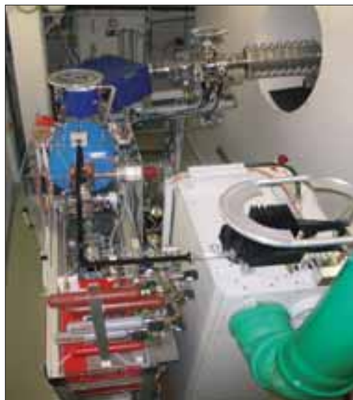
Fig. 6: New ion source platform: A rather unconventional layout of the new platform was necessary to fit it into the existing building
