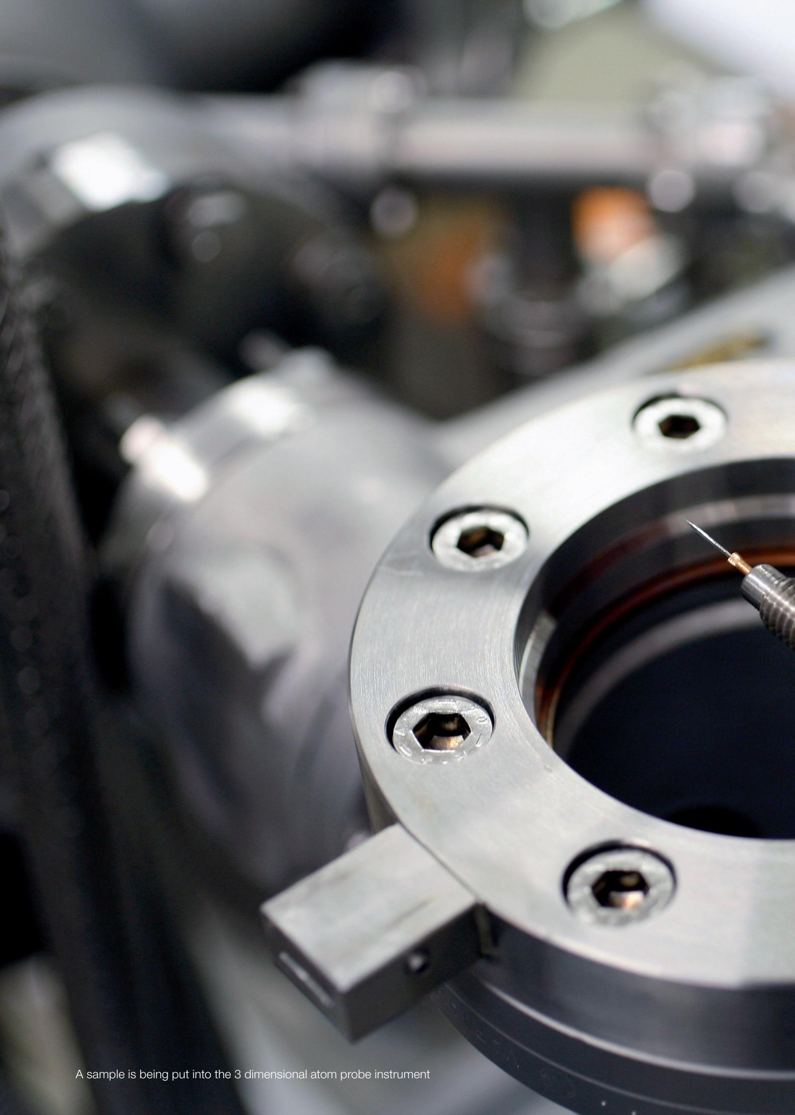
A sample is being put into the 3 dimensional atom probe instrument
