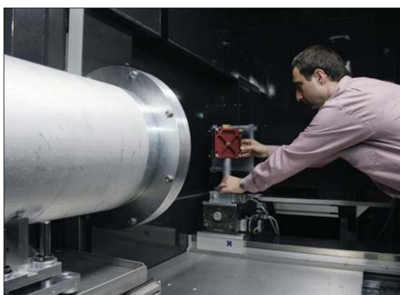
Preparing a fuel cell for tomographic imaging
