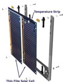
Fig. 1: Blow-up schematic diagram of the CIGSe thin film solar cell mini-module assembly as flown on Delfi-C3 (the temperature strip determines the temperature of the device).
