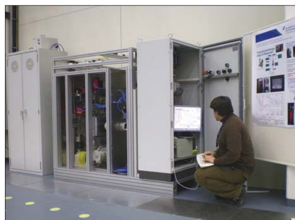
Fig. 3: Unique fully automated 10 kbar hydrogen gas-handling system for highest controlled gas pressures in combination with neutron investigations.
