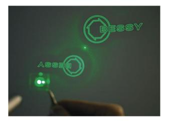
Diffractive optical elements (DOE) allow controlled manipulation of laser light by diffraction on microand nanostructured surfaces as well as an almost totally free shaping of light. That way, totally new optical functions can be realized that so far have been out of reach of classical optical components.
