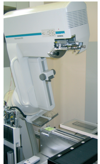
Fig. 4: Monochromator module with HOPG crystal attached to a conventional mammography unit
