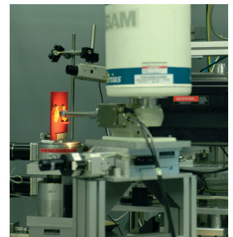
Fig. 4: Two cross-shaped pendants in the experimental set-up at the BAMline
