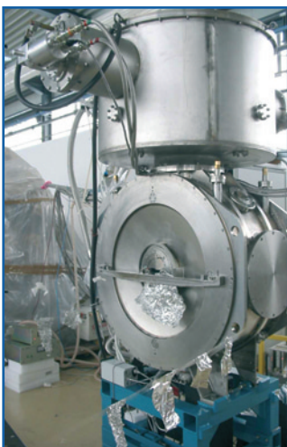
Fig. 5: Superbend prototype with B_{max} = 9.3 T
