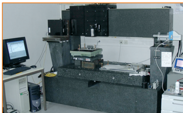
Fig. 1: The Nano-Optic Measuring Machine (NOM) in the optics laboratory
