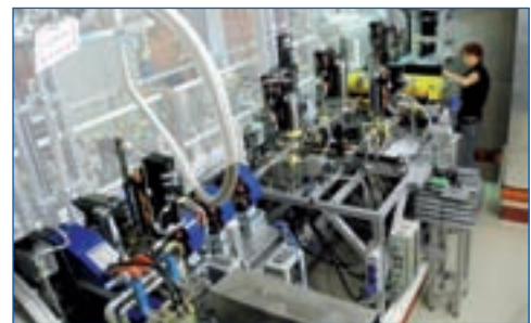
Fig. 12: Diagnostic beamline developed and installed by BESSY for the superconducting photoinjector at FZD. The RF cavity's cryomodule ends at the lower left corner of the picture.
