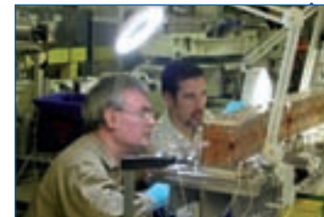
Fig. 7: Repair work of the septum magnets.
