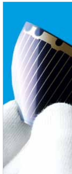
A flexible thin-film solar cell from HZB.
