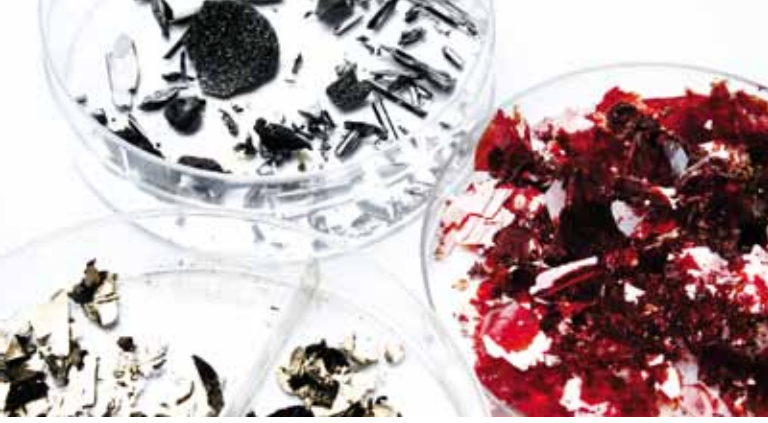
Artificially produced monocrystals of \text{CuInS}_2 (top left), \text{TaS}_2 (bottom left) and \text{PtS}_2 (right)
