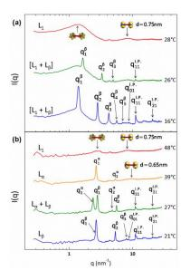
SAXS spectra of I2COSAN<sup>-</sup> anion self-assembled in water at 12.5 (a) and 59 (b) %v/v and at different temperatures (Bauduin et al, Angewandte Chem. Int. Ed.2013)
