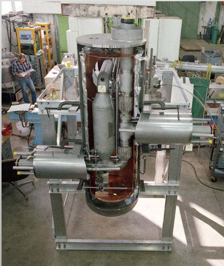
distribution box with heat exchanger
