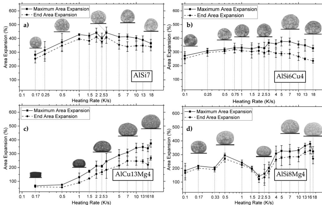
**Figure 1.** Maximum area expansion and end area expansion (measured during cooling at ~300 °C) as a function of the heating rate (logarithmic scale) applied to precursors of the alloys (a) AlSi7, (b) AlSi6Cu4, (c) AlCu13Mg4, and (d) AlSi8Mg4. Averages over all experiments carried out on a particular alloy are given. X-ray radioscopic images for one representative sample at the state of maximum expansion for the indicated heating rates are also displayed.
