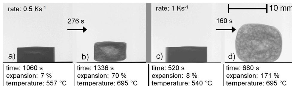
**Figure 2.** X-ray radiograms of foams after the first visible crack has been detected (a,c) and at the end of the heating ramp after 695 °C has been reached (b,d) at heating rates of 0.5 K/s (left) and 1 K/s (right).
