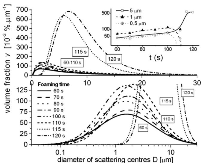
**Figure 2.** Pore size distributions  $v(D)$  in zinc foams. Upper: entire size range with inset showing volume fraction of scattering centres with  $0.5$ ,  $1$  and  $5 \mu\text{m}$  size as a function of time, lower: semi-logarithmic representation restricted to scattering centres with small volume fractions.
