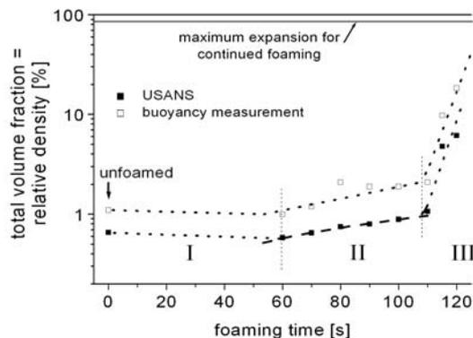
**Figure 3.** Total volume fraction of pores in foamed zinc as a function of foaming time at foaming temperature of 440 °C as determined by buoyancy measurement and USANS. The dotted lines are merely for orientation, whereas the dashed line represents a linear fit.
