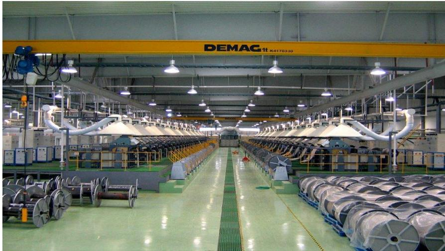
*Figure 11. Nickel foam production unit at the Inco Advanced Technology Materials, Dalian, China (Courtesy of V. Paserin).*
