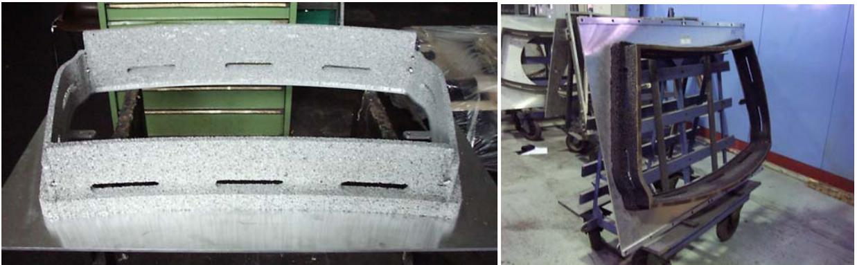
*Figure 8. Vacuum lifting tool for Pilkington containing an Alporas aluminium foam ring
