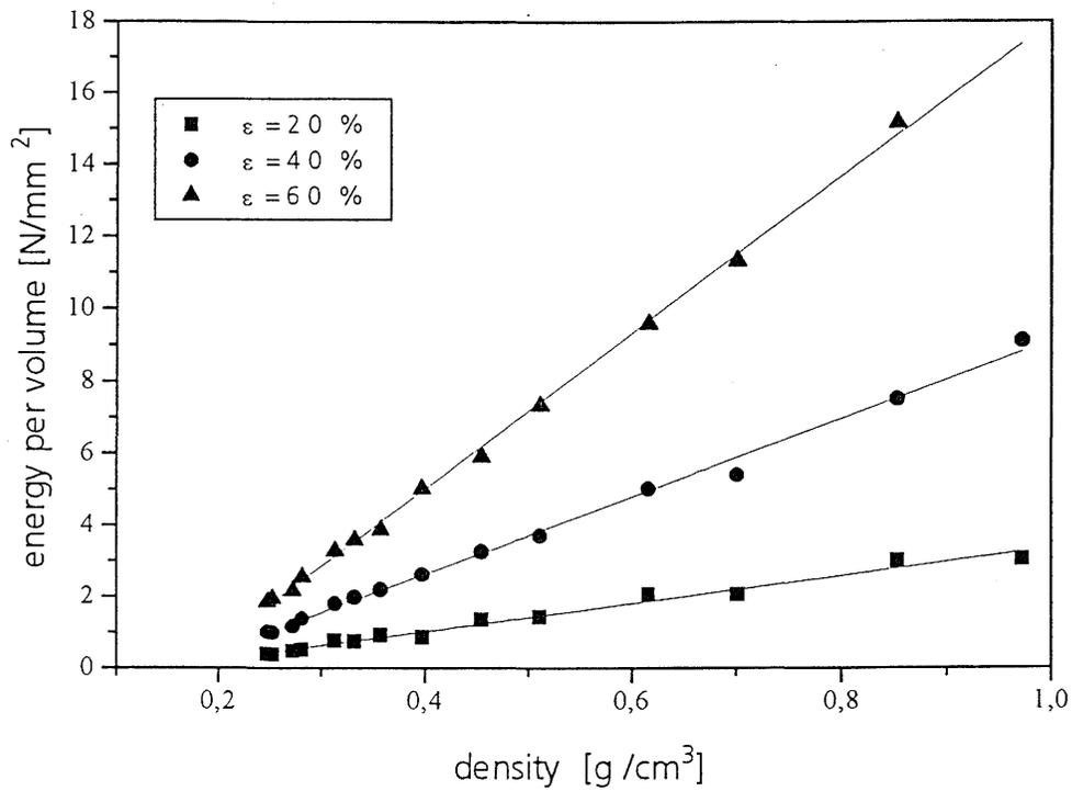
Fig. 4: Energy per unit volume absorbed by various AlSi12 foams after compression strains  $\epsilon$  of 20 %, 40 % and 60 %.
