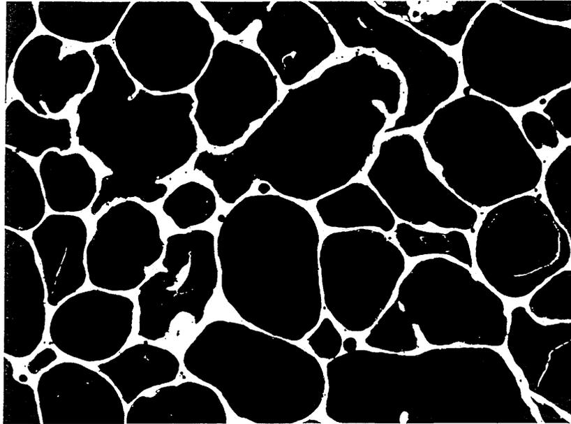
*Fig. 1: Cell structure of an aluminium foam (9:1)*
