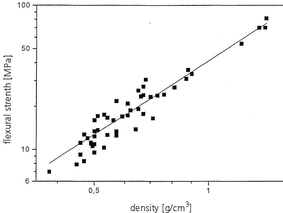
Fig. 2: Flexural strength of AlMg3 foams.
