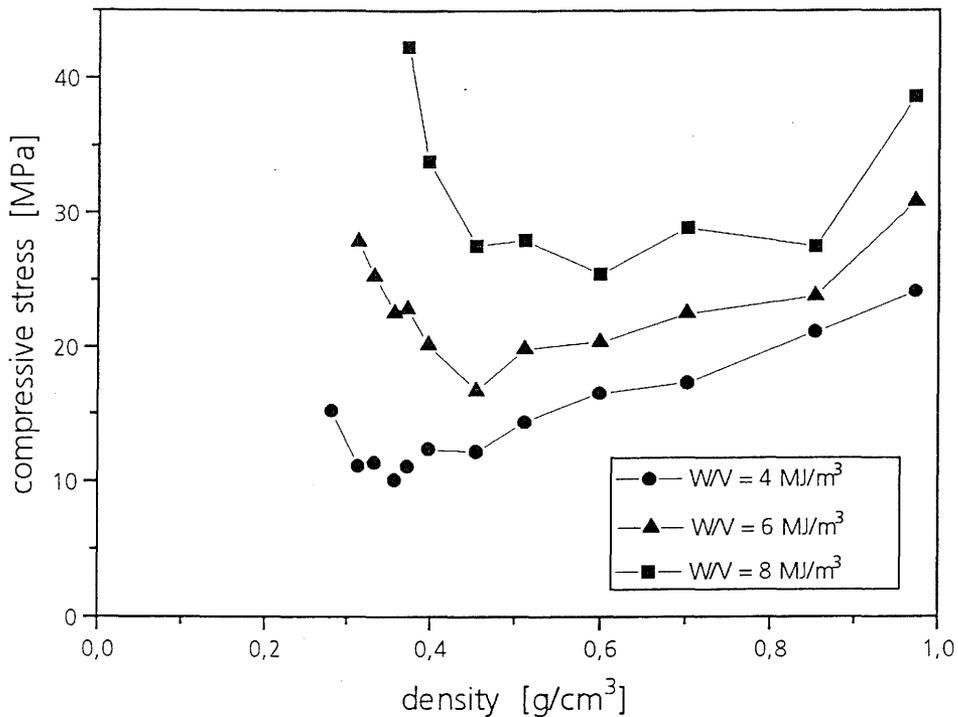
Fig. 6: Maximum stress occurring when a given deformation energy is absorbed by foams of various densities.
