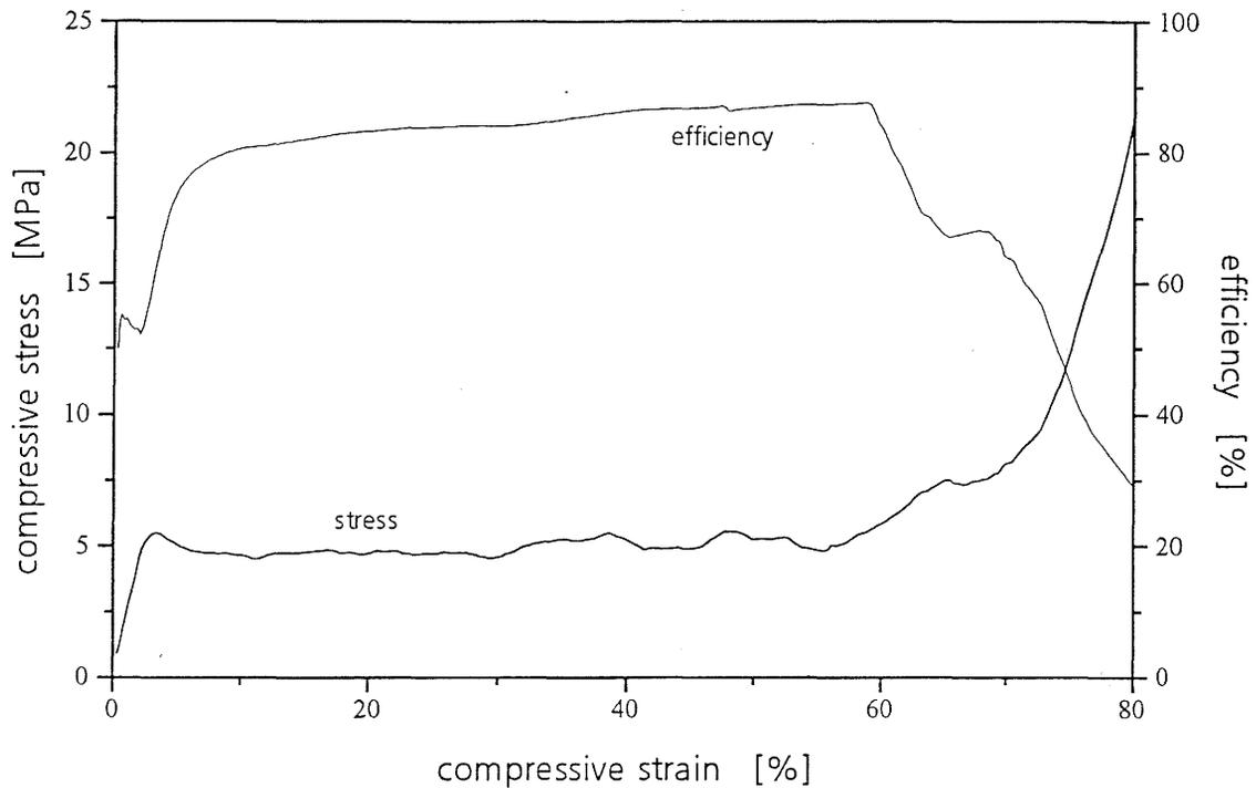
Fig. 3: Compression stress and energy absorption efficiency of an AlSi12 foam ( $\rho=0.36 \text{ g/cm}^3$ )
