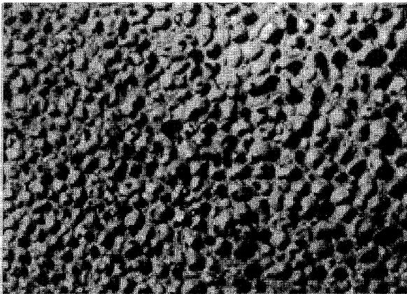
Figure 2: Typical structure of aluminum metal foam produced with powder metallurgy.
