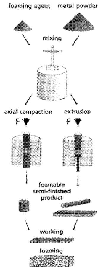
Figure 1: Schematics of processing steps for metal foaming by powder metallurgy.
