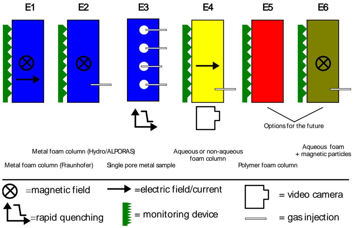
Figure 3: schematical description of the six planned experiments
