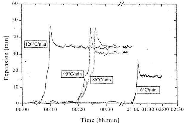
Figure 4: Expansion curves of 6061 samples containing 0.6 wt. %  $\text{TiH}_2$  for different heating rate.
