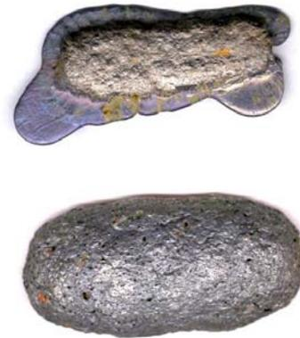
**Figure 5:** Lead foams made from two different lead powders. Upper: low-oxygen powder (0.06 wt.%), lower: higher oxidised powder containing 0.46 wt.% O [13].
