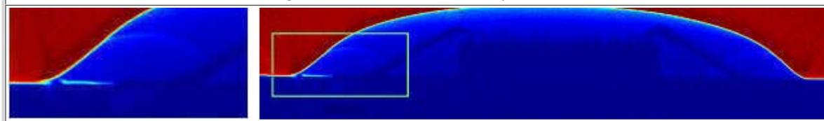
Fig 5c&d: Radioscopy with delamination between glob-top and circuit board: (c) detail, (d) overview
