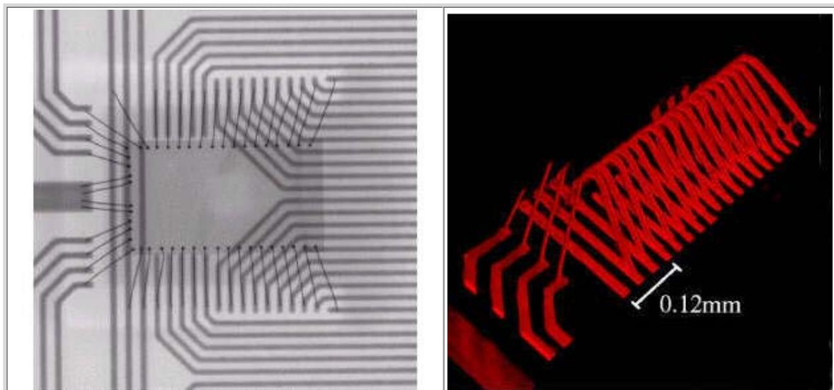
Fig 5a&b: Radioscopy image taken perpendicularly to the circuit board's surface (a), 3D-rendition of a tomographic reconstruction of the bonding wires and the metallization layer on the circuit board on a COB.
