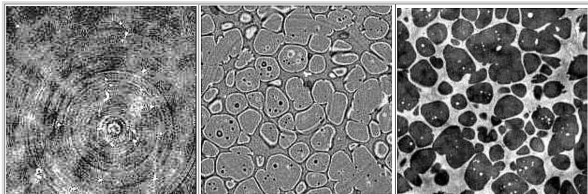
Fig 6: Three tomographic slices of an aluminium-silicon alloy quenched from the semi-solid state, obtained (a) using absorption contrast, (b) using phase contrast and a single propagation distance, (c) using phase contrast and holographic reconstruction based on four distances [4].
