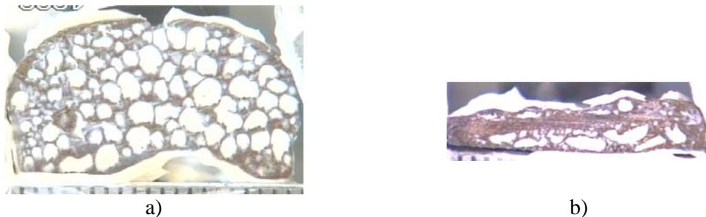
**Figure 7.** Lead samples processed under normal gravity conditions, foaming time 30s
