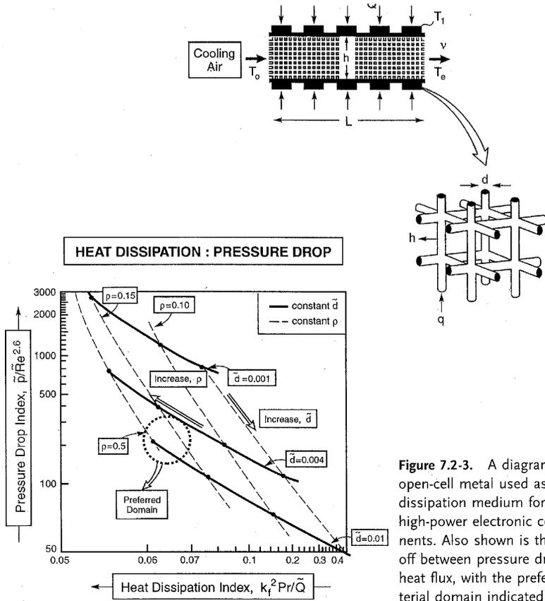
Figure 7.2-3. A diagram of an open-cell metal used as a heat dissipation medium for cooling high-power electronic components. Also shown is the trade-off between pressure drop and heat flux, with the preferred material domain indicated [7].
