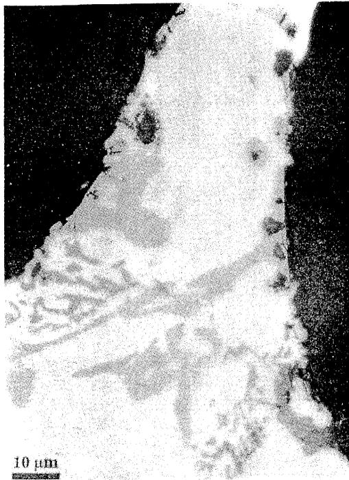
**Figure 7.** Microstructure of a foam made by injecting gas into a SiC reinforced melt („Alcan”-foam).
