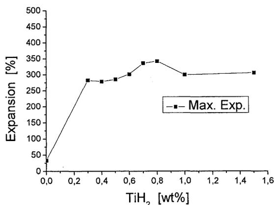
**Figure 5:** Expansion of route II AlSi6Cu4 foams as function of TiH<sub>2</sub>-contents, optimum at 0.8 wt%.
