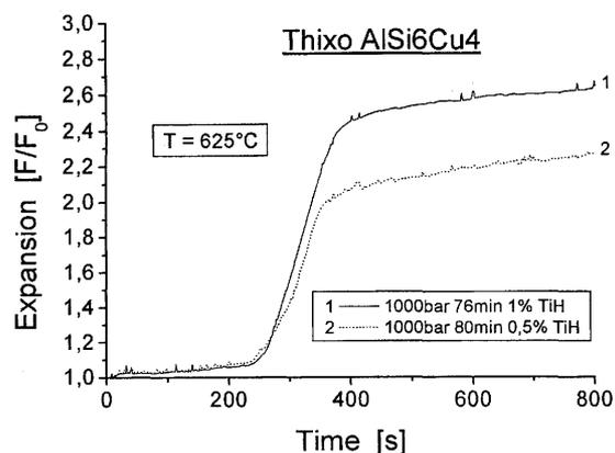
**Figure 6:** Expansion curve of thixo-cast precursors with different TiH<sub>2</sub> contents and slug heating time.
