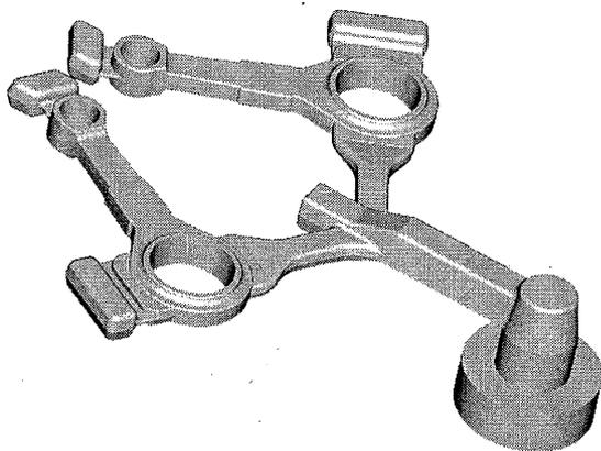
**Figure 4:** Component geometry used for the thixocasting experiments.
