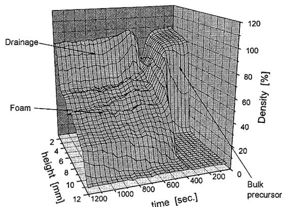
**Figure 8:** Foam density over time corresponding to sample 2 in fig. 6.
