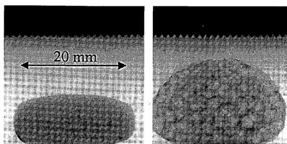
Figure 3: Radioscopic pictures of a route I precursor foamed in air under 8 bar (left) and under 1 bar (right),  $T = 600^\circ\text{C}$ .
