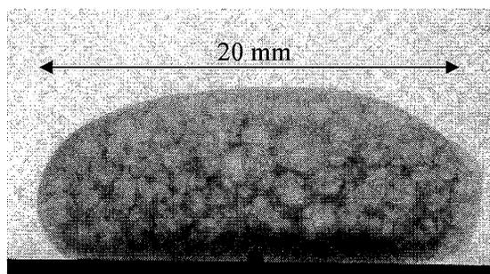
**Figure 7:** Radioscopic picture of a route II foam with strong drainage (sample 2 of fig. 6).
