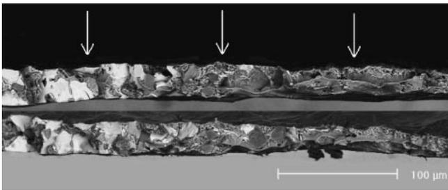
Fig. 4 Fracture surfaces of a cell wall width. Left arrow indicates cleavage of a  $\beta$ -AlFeSi plate. Middle arrow indicates fractured SiC particles and dimples with Si and the right arrow indicates ductile Al fracture. Upper fracture surface is mirrored for convenience.
