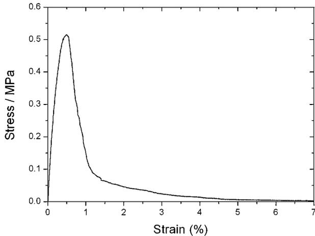
Fig. 3 Tensile stress-strain curve of the large foam sample ( $50 \times 50 \times 50$  mm) with 4.0% relative density.
