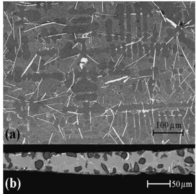
Fig. 2 (a) BSE image of an embedded and polished cross-section of a strut showing the microstructure. Dendrites of  $\alpha$ -Al and eutectic structure of Al-Si with needles of  $\beta$ -AlFeSi (white) (b) Embedded and polished cross-section of a cell wall. The dark inclusions are the SiC particles.
