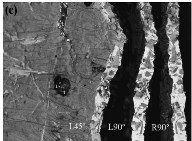
Fig. 6 (a) BSE image of the area marked by the black square in Fig. 5(a), prior to deformation. (b) After deformation, white arrow indicates the point of initiation. (c) Left fracture surface at  $45^\circ$  and  $90^\circ$  and the right fracture surface at  $90^\circ$ .
