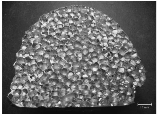
Fig. 1 Macrostructure of the metal foam made by the melt route.
