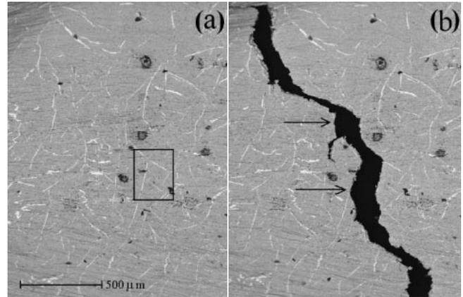
Fig. 5 (a) BSE image of the cell wall used in the *in-situ* tensile test prior to deformation. Black square indicates the area of Fig. 6. (b) Cell wall after deformation. Black arrows indicate initiation points.
