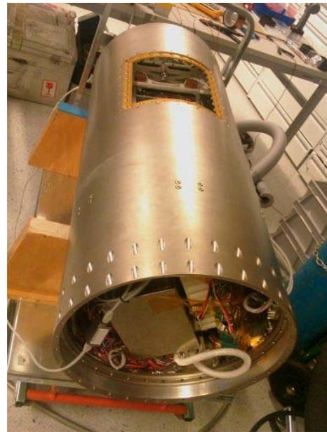
Figure 2. MASER 11 XRMON metal foam module
