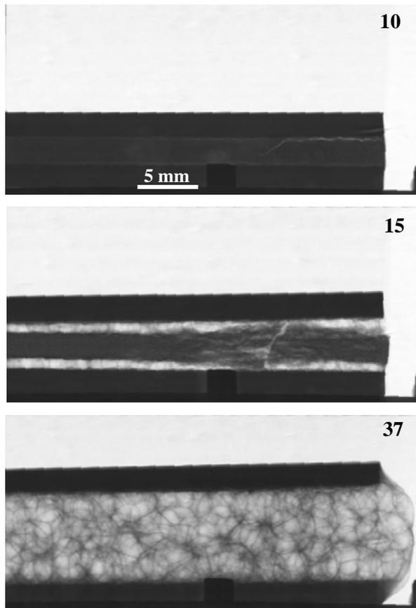
**Figure 2.** Series of radioscopic images of an expanding AlMn1/AlSi7-foam /AlMn1 – sandwich [8]. Foamed at a furnace temperature of 750°C.
