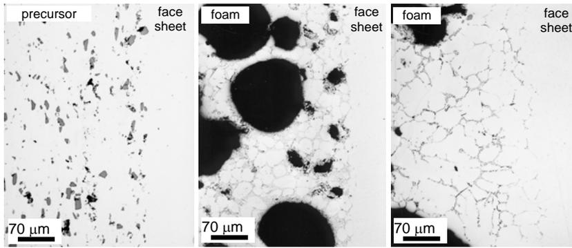
**Figure 3.** Metallographic images of sandwich structures with an AlSi7 core. Three different expansion stages are shown: left: unfoamed precursor material, middle: sandwich shortly before maximum expansion, right: sandwich at the onset of face sheet melting. The width of each image is 0.75 mm.
