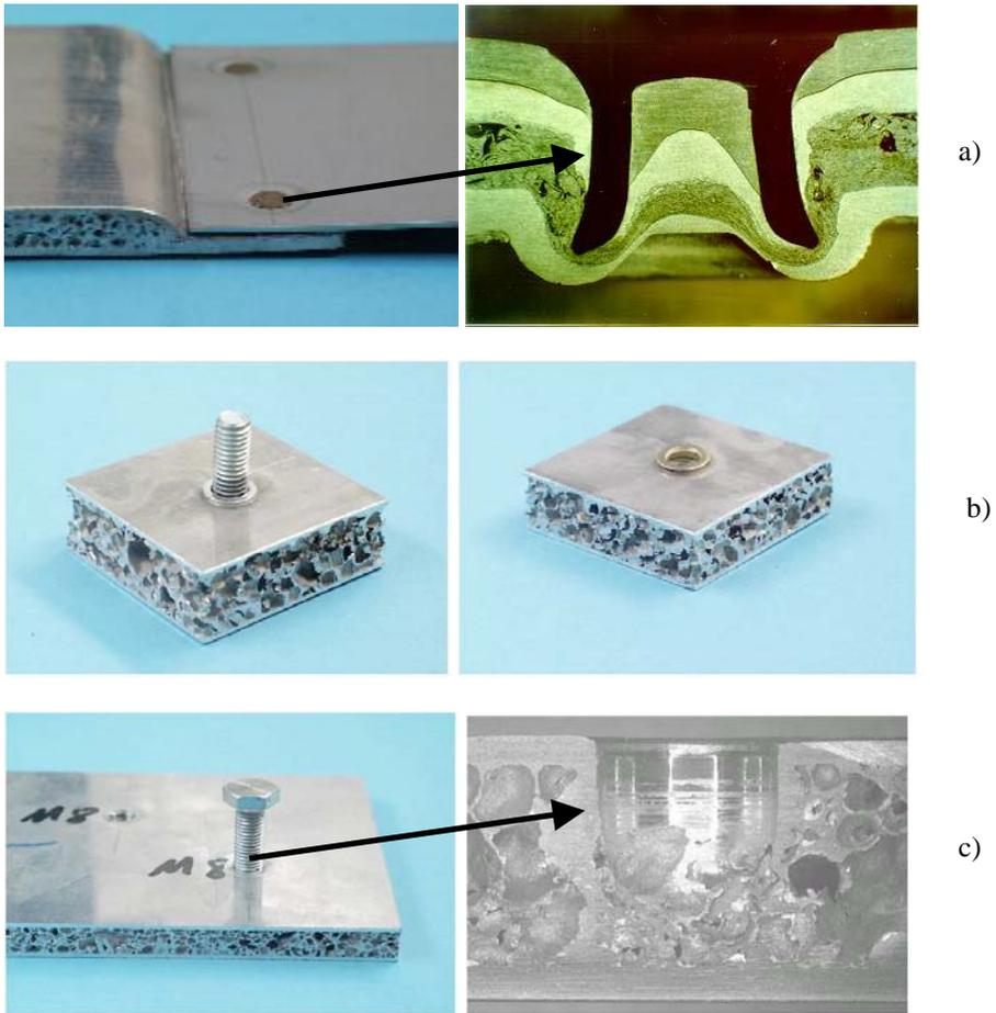
**Figure 8:** Different joining techniques for AFS. a) Punch riveting, b) Riveting nuts and screws, c) Flow drilling
