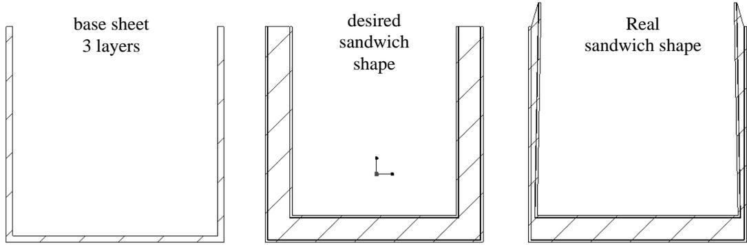
**Figure 6:** limitations of manufacturability of AFS
