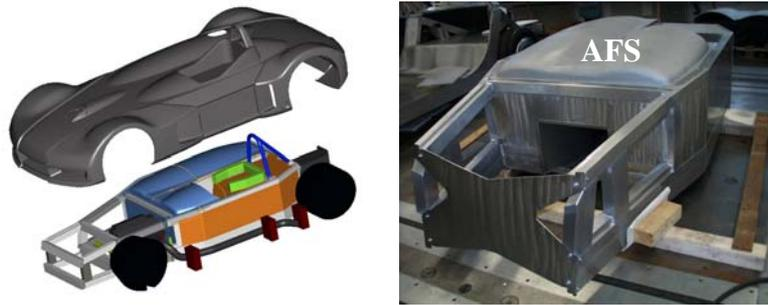
**Figure 5:** „EUROC 99“ concept racing car, left: CAD- Model of entire car, right: space-frame structure with AFS-parts.
