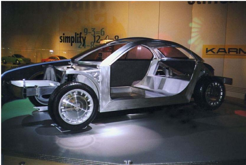
**Figure 4:** „Detroit Show Car 1998“ developed by Karmann (Osnabrück) for demonstrating potential uses of aluminium foam sandwich panels. The rear bulkhead and the front firewall (not directly visible) are made of AFS.
