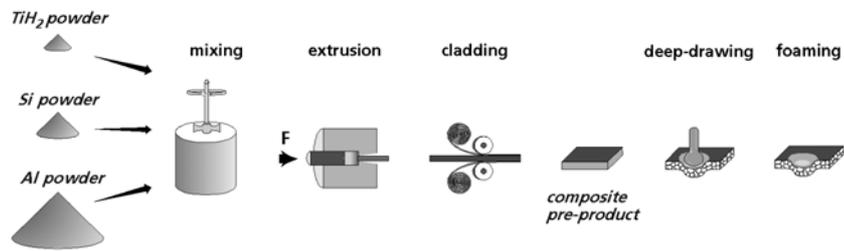
**Figure 1.** Process steps for making sandwich panels with aluminium foam cores.
