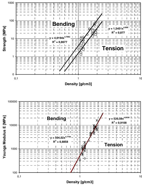
**Figure 8:** Strength and Young's Modulus as a function of density obtained from bending and tension tests [13].
