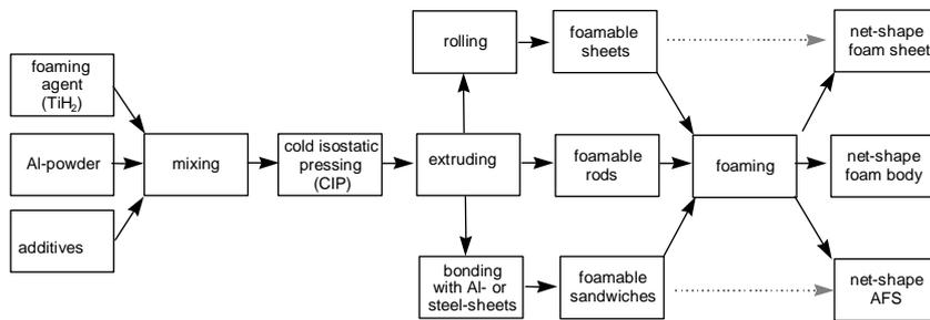
**Figure 1:** Foam production by powder compact foaming technique
