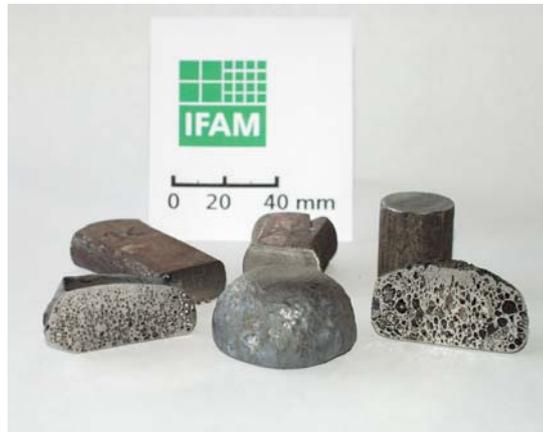
**Figure 9:** Iron foams obtained from the blowing agent process
