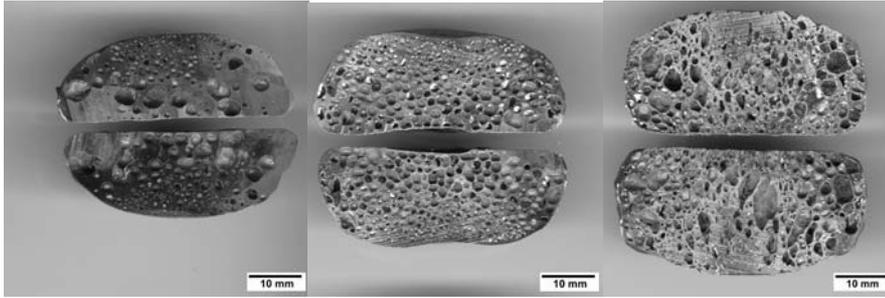
**Figure 10:** Iron-based metal foams made from extrusion pressed powder mixtures of Fe + 2,5% C. Left: 0,0% SrCO<sub>3</sub>, middle: 0,25% SrCO<sub>3</sub>, right: 0,50% SrCO<sub>3</sub>
