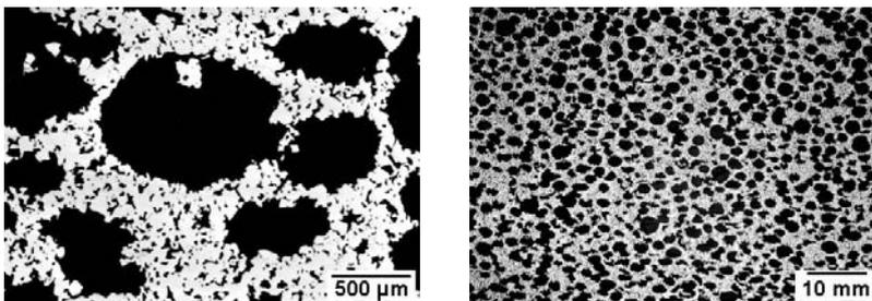
**Figure 7:** Pore structure of open porous Titanium with 67% Porosity.
