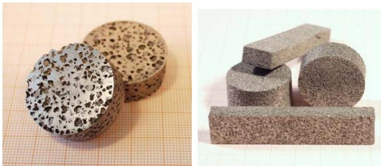
**Figure 6:** Open porous Titanium made by space holder technique. Left: Pore size 1-4 mm, right: pore size approx. 500 $\mu$ m, Porosity 55-80%.
