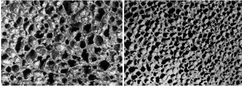
**Figure 5:** Zn and Pb-foam (width of images is about 5 cm)
