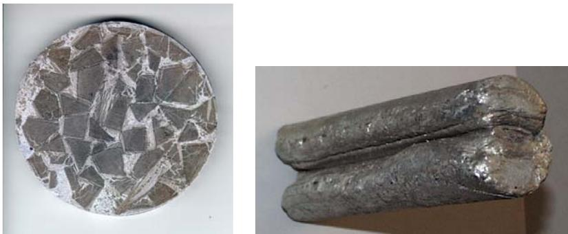
**Figure 4:** Left: aluminium foam part made by inserting various pieces of foamable material into the mould. Right: foam part made of two pieces of precursor without achieving bonding between the two pieces.
