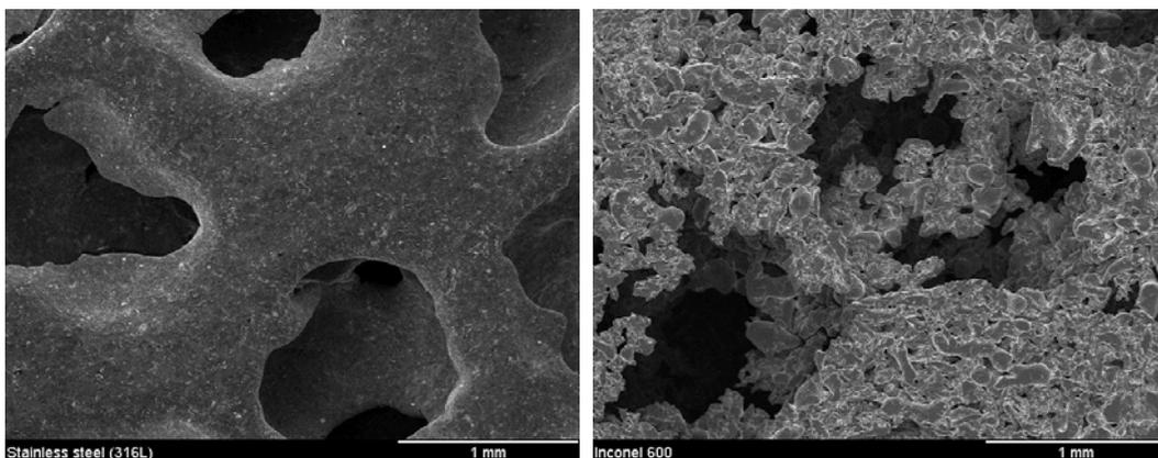
**Figure 12:** SEM images of sintered specimen. Left: stainless steel 316L, 1100°C, 1h, particle size  $16 < \mu\text{m}$ . Right: Inconel 600, 1250°C, 1h, particle size 100-200  $\mu\text{m}$ . [17]
