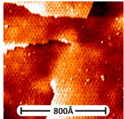
Scanning tunneling microscopy shows the topography of graphene on gold with periodic beatings ten times larger than the periodicity of the carbon atoms. These beatings are moiré-patterns, emerging because of the different atomic structures of graphene and the underlying monolayer of gold atoms. The structure of moiré influences chemical interactions between gold and graphene layer and also electronic properties and spin behavior in graphene.
