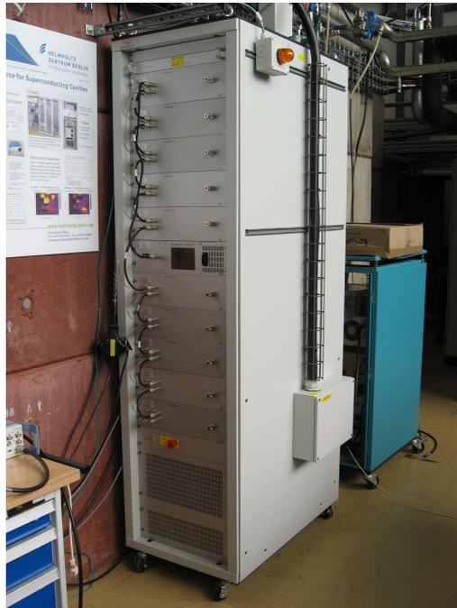
**Figure 3.23:** Solid state transmitter (1.3 GHz 15 kW) at the HoBiCaT test facility of the HZB.
