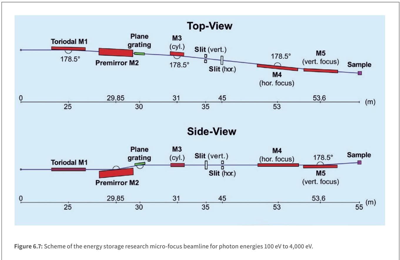
Figure 6.7: Scheme of the energy storage research micro-focus beamline for photon energies 100 eV to 4,000 eV.
