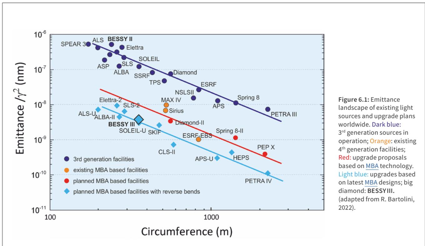
This new light source must support the scientific focus fields described in Chapter 4 and must be within the parameter ballpark of worldwide discussed upgrades of SR-facilities depicted in Figure 6.1. Such a globally competitive soft-to-tender X-ray large-scale facility can only be realized as a green-field facility complementing the surrounding WCRC campus environment of the HZB in Berlin-Adlershof.
