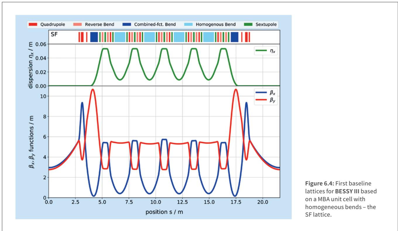
Figure 6.4: First baseline lattices for BESSY III based on a MBA unit cell with homogeneous bends – the SF lattice.
