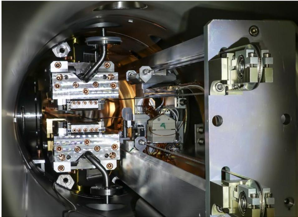
Figure 6.5: View inside the [CPMU17](#) during the magnet field measurements. The magnet structure on the left side and the in-vacuum measurement bench on the right side are shown.
