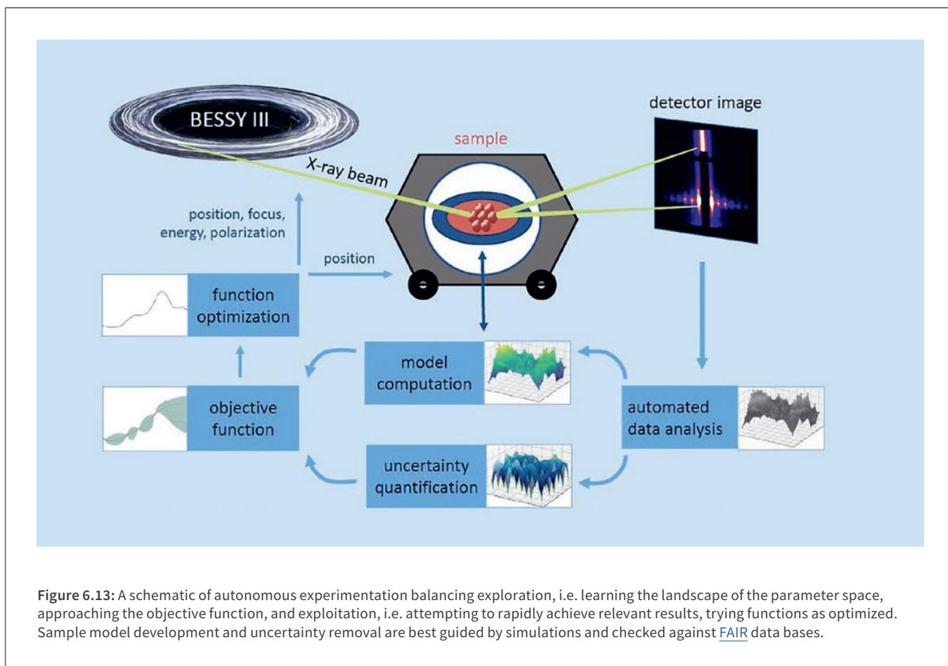
**Figure 6.13:** A schematic of autonomous experimentation balancing exploration, i.e. learning the landscape of the parameter space, approaching the objective function, and exploitation, i.e. attempting to rapidly achieve relevant results, trying functions as optimized. Sample model development and uncertainty removal are best guided by simulations and checked against FAIR data bases.
