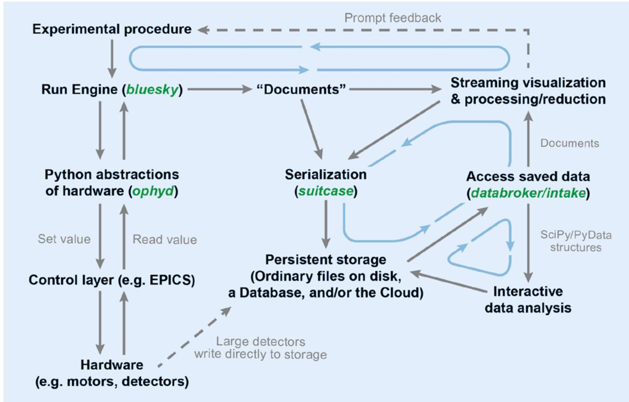
Figure 6.12: Sketch of the automation framework Bluesky<sup>[109]</sup> as a rich experiment control software ecosystem. Features include ophyd, a device abstraction layer overcoming the flat EPICS data model, bluesky, a run engine covering experiment design, data acquisition, -analysis and -handling flow control and databroker, providing native connectivity to nearly any extending python based scientific toolkit.
