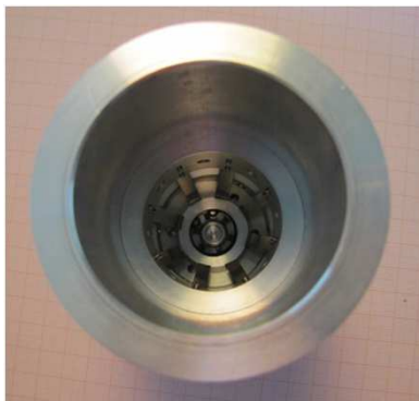
Look inside: Position of puck with photocathode
