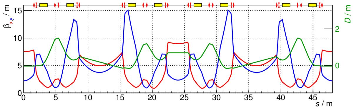
Figure 1.3: MLS magnet optics for standard user operation: Horizontal (red) and vertical (blue)  $\beta$ -functions  $\beta_{x,y}$  as well as horizontal dispersion  $D$  ( $\beta_{x,y}$ ) were measured by fitting a model to the orbit response matrix (LOCO [26]). The top axis indicates the position of dipole (yellow) and quadrupole (red) magnets.
