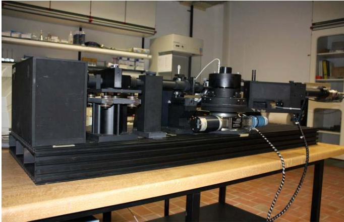
Dynamic light scattering instrument, manufactured by ALV
