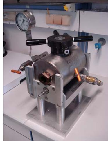
Summary of experimental findings (d-spacings) for the oligolamellar DMPC bilayers film against excess water ( $D_2O$ ), left. Note that the lipid film irreversibly detaches from support after crossing the phase boundary of the corresponding bulk system at 69 MPa and 38 °C. Photograph of the high pressure cell for neutron reflectometry (right).<sup>6</sup>
