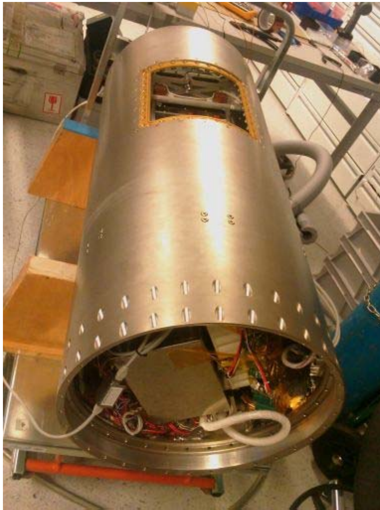
Figure 5: XRMON module for metal foams assembled and ready to fly
