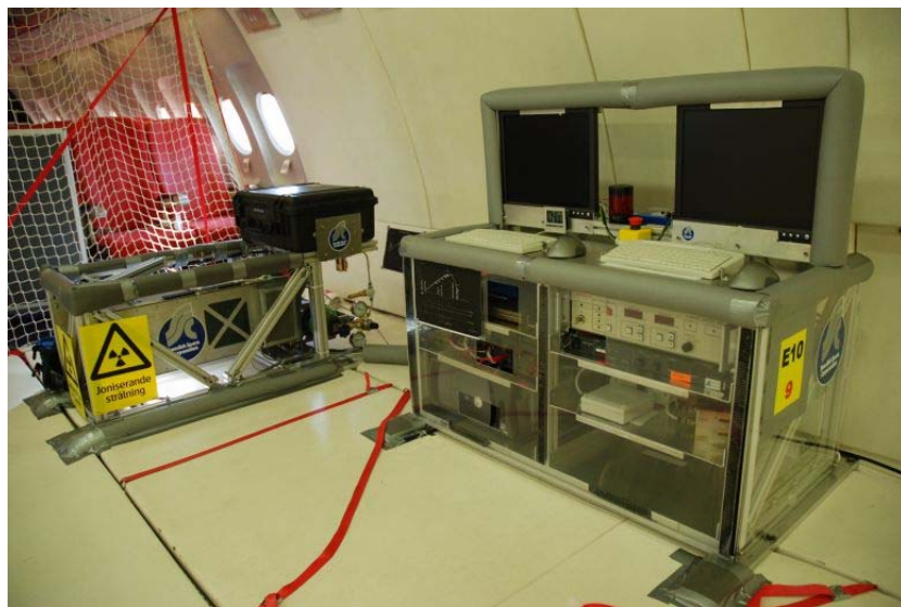
Figure 1: X-ray scanner with attached black box with 6 exchangeable metal foaming furnaces and control pool adapted for the PFC
