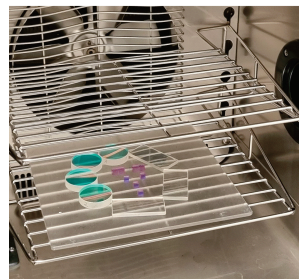
Fig. 6: Left – Samples in front of Co-60 source at HZB. Middle – Thermal cycling test sequence. Right – Alexandrite crystals in climate chamber at Altechna. Figures from [5].
