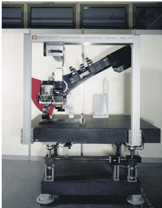
Fig. 3: Multipurpose diffractometer for residual stress-, texture and microstructure analysis at BESSY [2].
