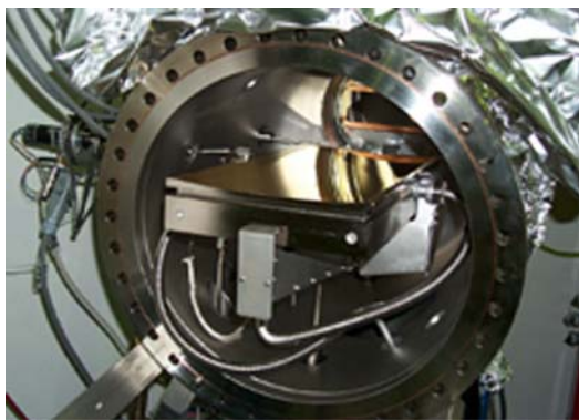
Fig. 2: Focussing mirror, cooling facilities and mechanics installed in the new vacuum chamber.
