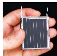
Fig.3: Encapsulated \text{CuInS}_2 -based monolithically integrated test module
