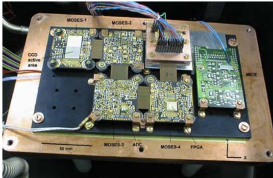
Fig. 1: MOSES detector electronics mounted inside the thermal vacuum chamber for functional tests and performance measurements after proton irradiation.
