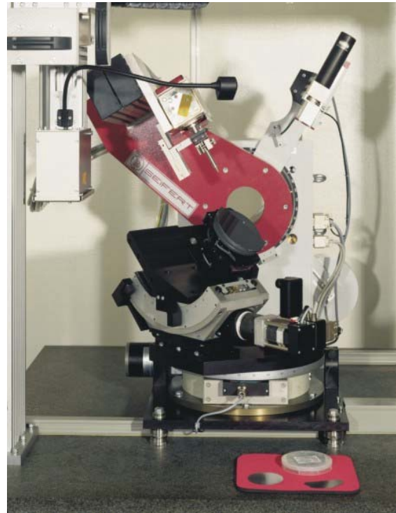
Fig. 1: The 5-circle diffractometer XRD 3003 ETA for the analysis of steep near-surface gradients of residual stress, texture and microstructure [1].
