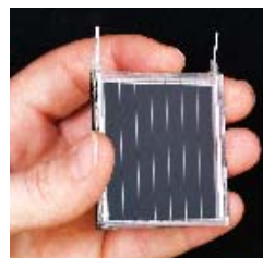
Fig.3: Encapsulated \text{CuInS}_2 -based monolithically integrated test module
