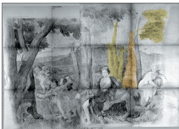
Fig. 3: Nicolas Poussin, Replica, Armida abducts the sleeping Rinaldo , 1 st neutron autoradiography assembled from 12 image plate records: In order to investigate the whole picture, two separated irradiations were carried out and finally recomposed.
