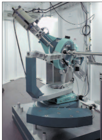
Fig. 3: MAGS, the new instrument for resonant magnetic scattering operated by the Hahn-Meitner-Institut at BESSY
