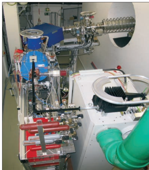
Fig. 6: New ion source platform: A rather unconventional layout of the new platform was necessary to fit it into the existing building
