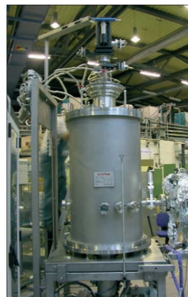
Fig. 2: The new ultra high vacuum high magnetic field reflectometer at UE46 PGM, BESSY
