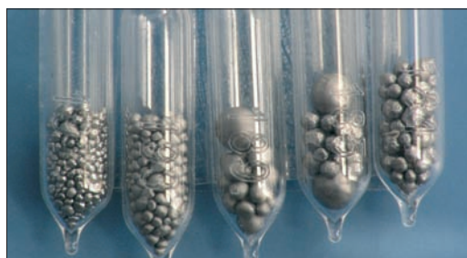
Fig. 1: Granules of pure Silicon enclosed in ampoules made of highly pure silica
