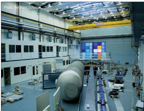
Photo: Bernhard Schürjan Neutron Guide Hall II in December 2006. The magnet will be placed in front of the big window at the end of the hall. The blue tubes on the right hand side are the neutron guides of the instrument EXED that will be operated with the magnet.
