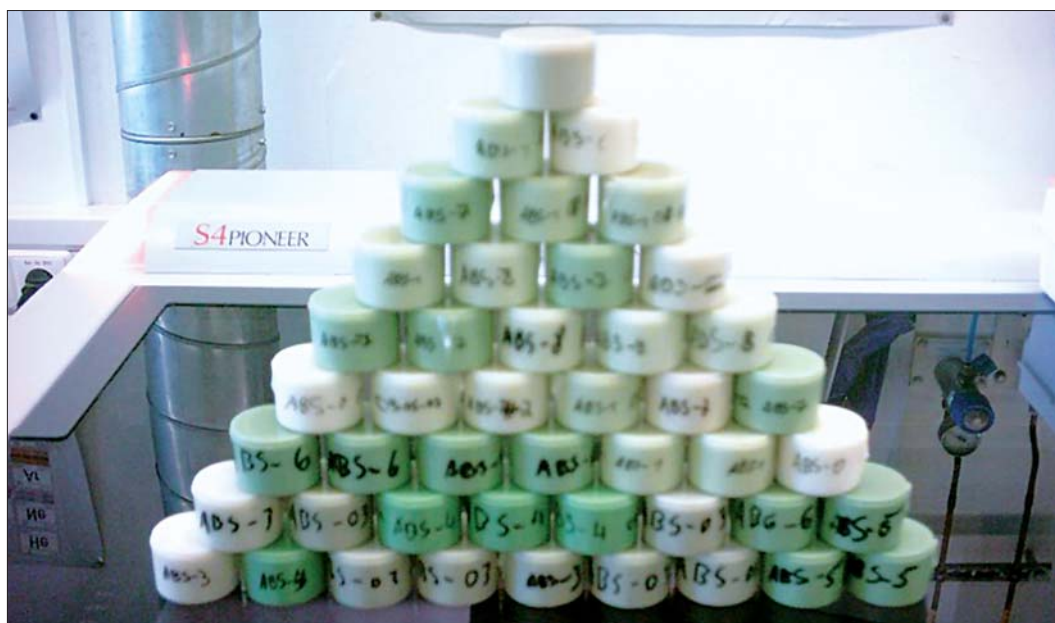
Fig. 3: Produced ABS standard Materials (solid bodies) containing the regulated Elements Pb, Br, Hg, Cr, Cd
