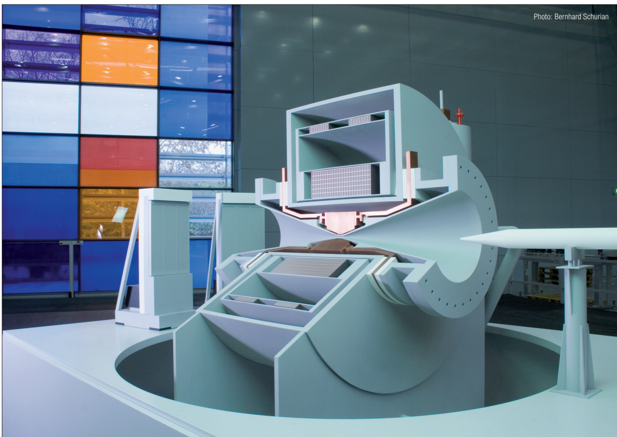
Model of HMI's new high field magnet. The model is cut open showing the inner design of the magnet.
